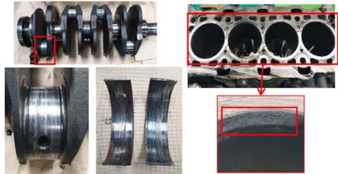
< Excessive wear of moving parts >
