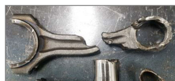
< Connecting rod broken >
