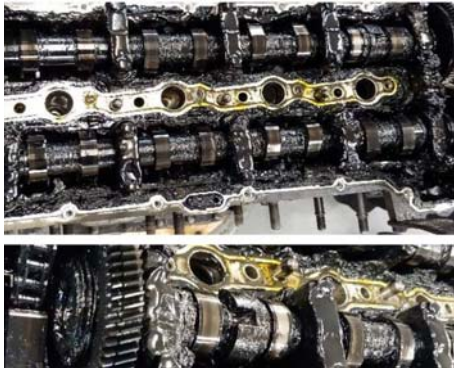
< Contaminated and gelled engine oil >
