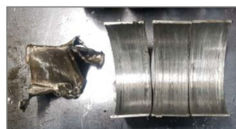
< Connecting rod bearing seizure >
